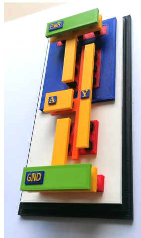
IHP130 Inverter with false power rails
