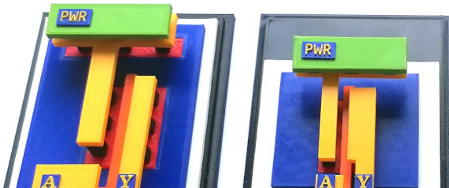
IHP130 Inverter with false power rails
